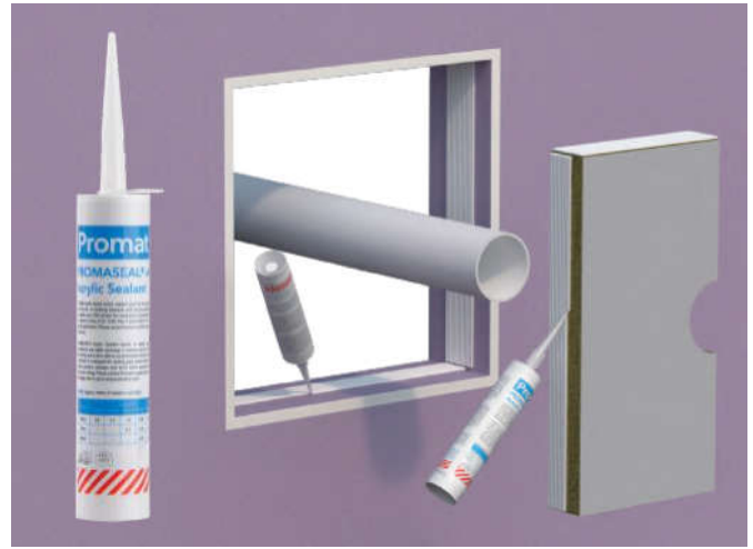
2. Apply PROMASEAL®-A Acrylic Sealant to the cut surface and the mating substrate.
