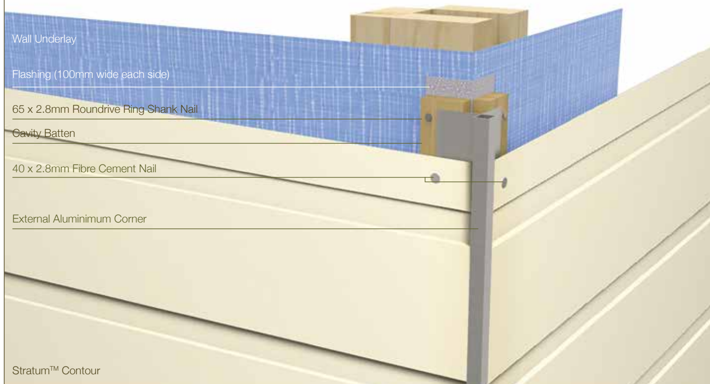
FIGURE 23 STRATUM™ CONTOUR - ALUMINIUM BOX CORNER
