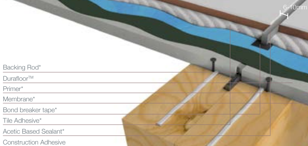
FIGURE 17 CONTROL JOINT WITH TILES
