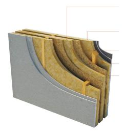
Wall width: 240mm (min) between inner faces of wall linings. 50mm (min) gap between studs (must not be bridged by any diagonal bracing).
