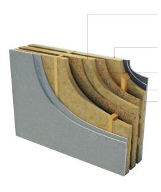
Wall width: 240mm (min) between inner faces of wall linings 50mm (min) cavity (gap between wall panels) 68mm (min) between stud frames
