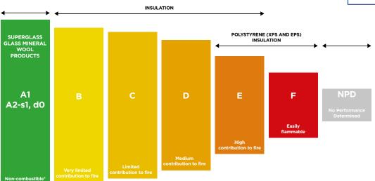
\*As set out in changes to the building regulations 2010 which bans the use of combustible materials, limiting the use of materials to those that achieve A1 or A2-s1,d0 on buildings in scope of the ban [as defined in regulation 7(4)]
