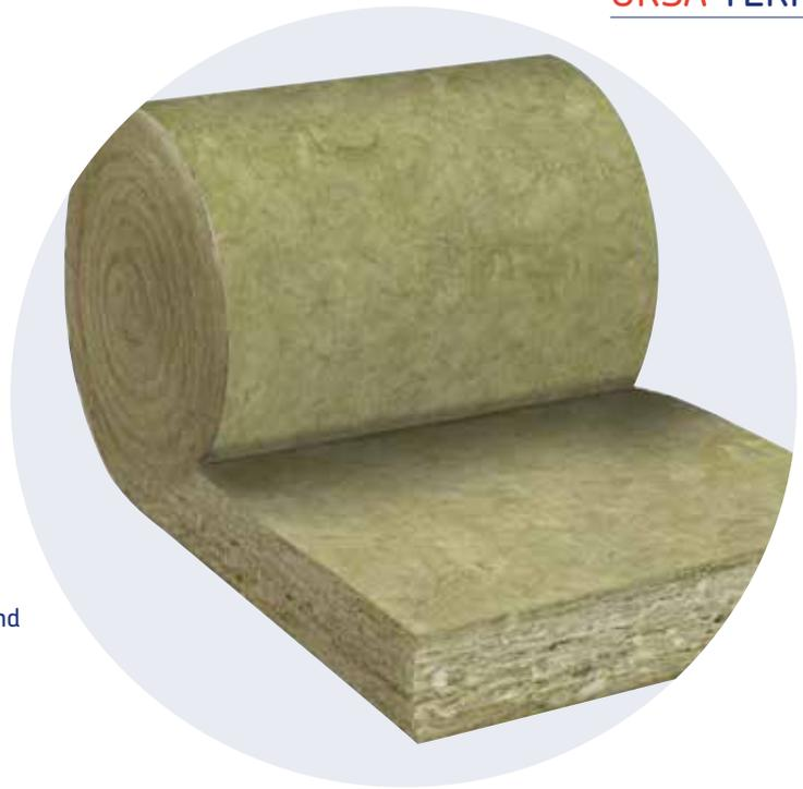
**URSA FRAMETEC** is a lightweight, non-combustible, glass mineral wool product. It is suitable for use in both timber and metal framed walls. **URSA FRAMETEC** has a thermal conductivity of 0.032 W/mK or 0.035 W/mK.
