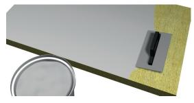
Apply above mentioned wet film thickness (final dry film thickness ≥ 0,7 mm) and consider drying time; If mineral wool boards are not pre-coated, ensure during installation the final dry film thickness on surface of ≥ 0,7 mm.
