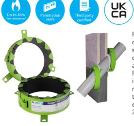
PipeBloc<sup>®</sup> PCP Collars are designed and tested to seal service penetrations in apertures containing combustible services and on bunches of cables. PipeBloc<sup>®</sup> PCP utilises specialist intumescent technologies which result in the collar expanding in the presence of heat or fire. This expansion is fast acting and up to 25 times the original size.
