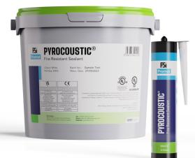
Pyrocoustic<sup>®</sup> Fire Resistant Sealant is a water based, acrylic sealant used to reinstate the fire resistance of wall and floor constructions in both linear joints and where apertures are penetrated by multiple services.
