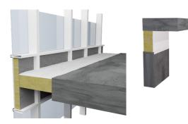
Flexi Coat<sup>®</sup> Fingers are made up of an 80kg mineral wool which has a lamella core to give it enhanced flexibility, and the Flexi Coat® Coating applied to it is able to flex and mould to accommodate this. Built up vertically, the blocks of mineral wool can be adapted to meet the different movement requirements of fire stopping seals, as well as curtain wall and perimeter façade applications.
