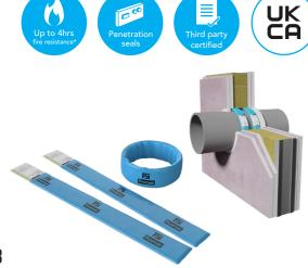
PipeBloc<sup>®</sup> PWP is a pre-cut wrap, designed and tested to seal service penetrations in apertures containing combustible plastic pipes and pipes with insulation. The expanding wrap reinstates the void left by combusting materials, exerting a pressure on the surrounding substrate to uphold the fire resistance of the compartment.
