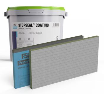
Stopseal® Batt is stone wool board coated with Stopseal® Ablative Coating. It's used to reinstate the fire resistance performance of wall and floor constructions, where apertures are penetrated by single or multiple services. The Stopseal<sup>®</sup> Batt is a high performance product making cutting and installation simple and swift.
