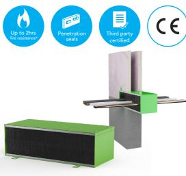
Pass-It<sup>®</sup> Transit System is a pre-assembled, intumescent device ETA-23/0076 encased in a 2 part steel shell, designed to prevent the passage of fire between compartments. Pass-It<sup>®</sup> Transit System allows for multi-service penetrations, where there is a requirement to change the service on a regular basis or allow for the provision of future, unknown, services.
