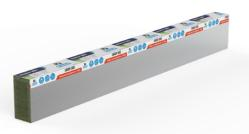
For use in open state cavities within the external building facade where continuous ventilation and drainage is required. Silverliner incorporates a foil lined mineral wool fibre board with a high-performance intumescent strip, so in the event of a fire the intumescent strip quickly swells to close the gap, slowing the spread of smoke and flame around the outside of a building.
