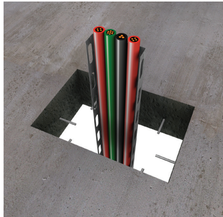
2. For building penetration seals in floors, install 100 mm plugirons. These plug irons should be installed central of mortar penetration seal every 300 mm, but minimum one plug iron on each side and should be inserted the floor 50 mm and covered by 50 mm with PROMASTOP®-M. No plug irons required for wall application.
