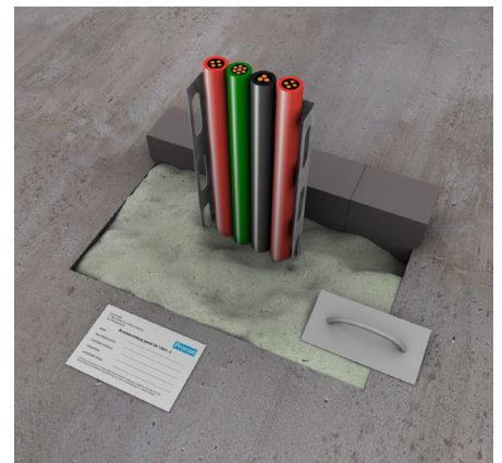
6. Smoothen the surface; Fix identification label
