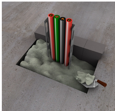
5. Close remaining opening with PROMASTOP®-M. Consider that mortar is sagging in bigger penetration sizes, which requires a work over to reach correct thickness or height;
