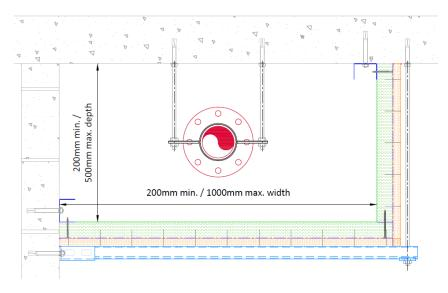
For horizontal enclosures, supports are required at 1200mm intervals via metal strut C-sections, 41x41x3mm thick.
