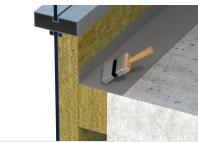
5. Apply correct thickness of PROMASEAL®-A spray onto the mineral wool with overlapping on the vertical facade insulation and the floor
