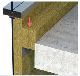
3. Compress mineral wool and insert in the joint.
