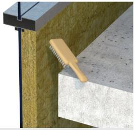
1. Clean aperture opening and dampen with water if required.
