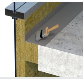
4. Apply correct thickness of PROMASEAL®-A spray onto the mineral wool with overlapping on the vertical facade insulation and the floor.
