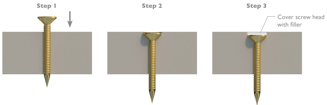
Figure 8 Fixing steps
