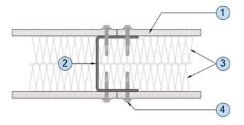
1: 9.5mm DURASTEEL® 2: 80mm x 60mm x 3mm CRC's at 1200mm centres 3: 2 layers, 40mm x 45kg/m<sup>3</sup> Stone Wool 4: M5.5 x 38mm Self-drill, Self-tap TEK Screws at max 200mm centres
