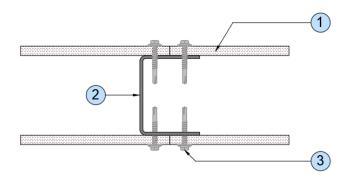
1: 9.5mm DURASTEEL® 2: 80mm x 60mm x 3mm CRC's at 1200mm centres 3: M5.5 x 38mm Self-drill, Self-tap TEK Screws at max 200mm centres
