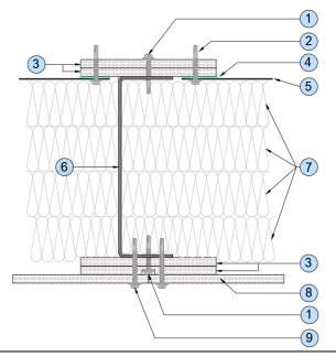
1: M5.5 x 38mm Self-drill, Self-tap TEK Screws at max 600mm centres
