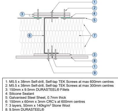
9: M5.5 x 38mm Self-drill, Self-tap TEK Screws at max 200mm centres
