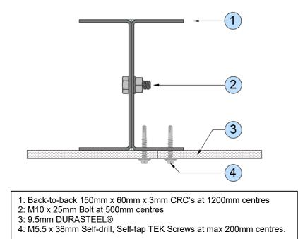
The maximum span of the self-supporting ceiling assembly is 4400mm. The width of the ceiling assembly is unrestricted.
