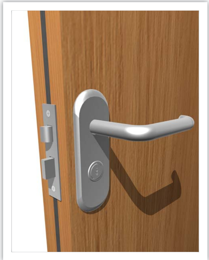
Detail 4 Intumescent strips interrupted by hardware not suitable for doors expected to perform beyond 30 minutes
