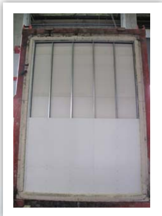
Promat partition system test
