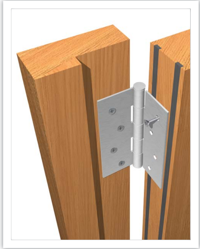
Detail 2 Intumescent strips interrupted and continuous in leaf only
