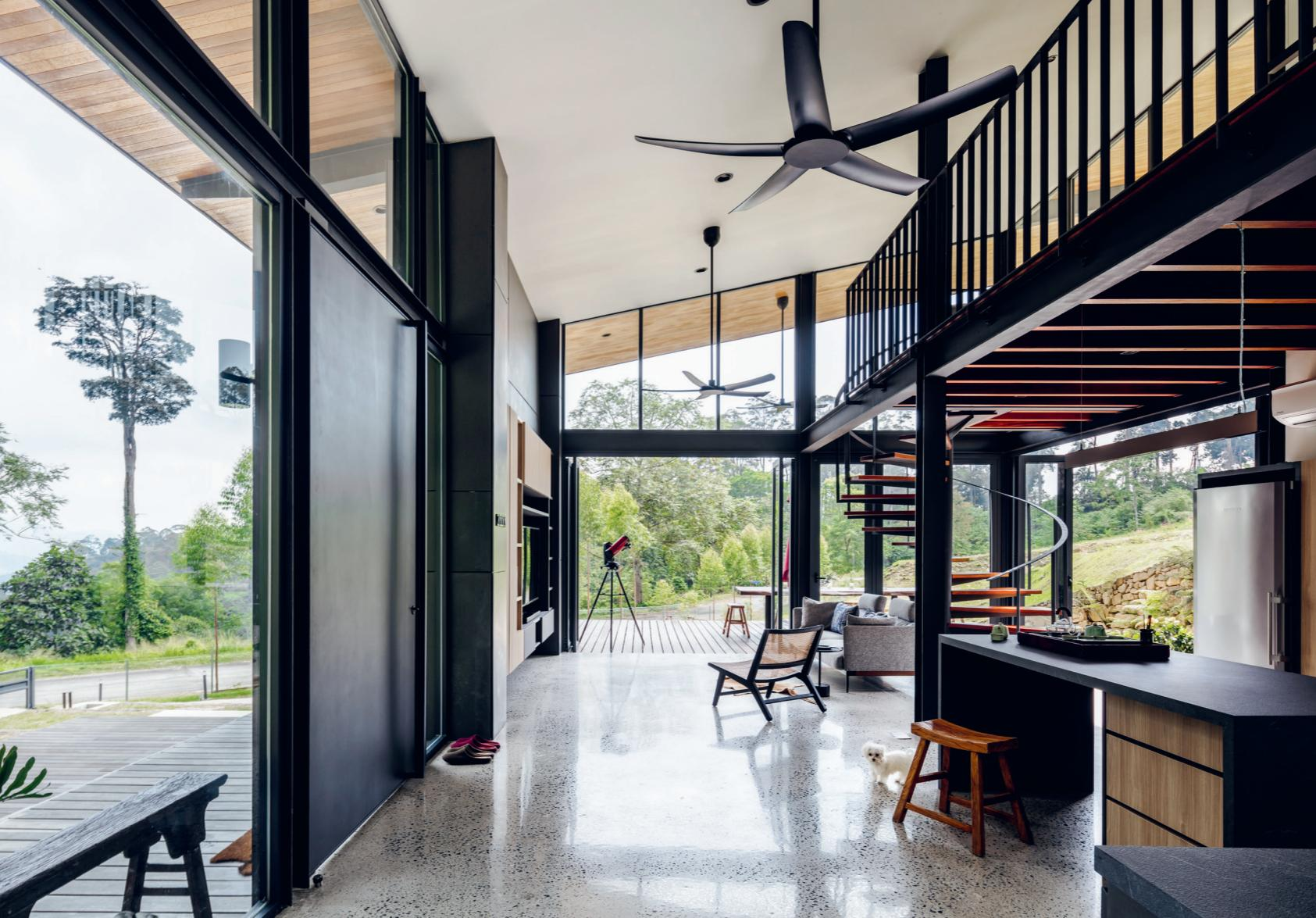
The architects consciously decided on a design that allows natural ventilation and does not require air conditioning. The positioning of the building and the size of the openings allow it to be well cross-ventilated.
