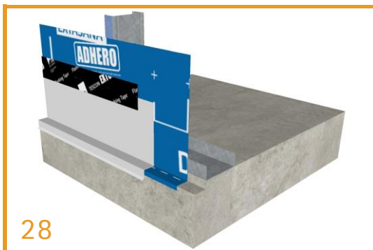
Slab Step Down - Edge Base Detail Connection ADHERO is finished by adhering onto the concrete edge (using ORCON® CLASSIC if necessary). The flashing is fixed with a self-taper and over taped.
