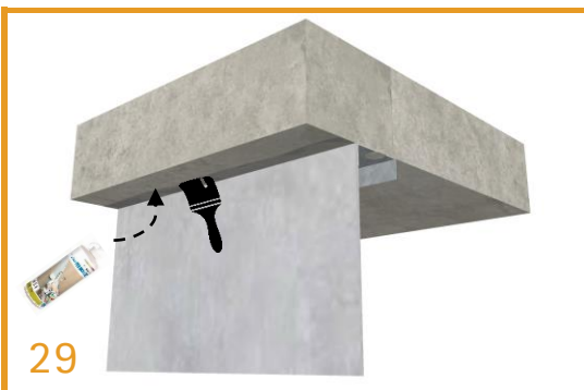
Preparing The Soffit Porous concrete or masonry may need to be primed with TECON® PRIMER RP using a brush.
