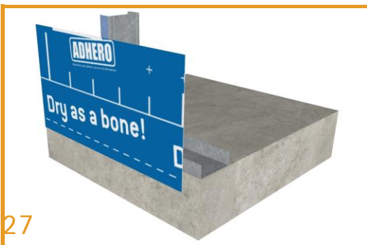
Connect to Straight Slab Edges ADHERO is finished by adhering it onto the concrete edge. Use ORCON® CLASSIC if necessary as per step 26..
