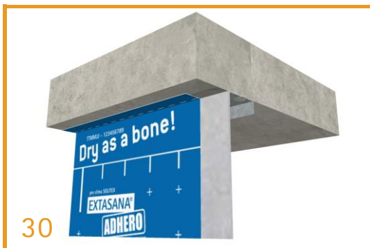
Weatherproof Seal to Soffit SOLITEX EXTASANA ADHERO® is applied to overlap onto the soffit by at least 30mm ensuring it does not protrude past the proposed finished cladding surface.
