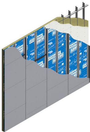
Isometric view of single layer top hat construction
