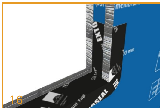
Window Wet Seals – Front & Back Seal TESCON® ADHISO WS is applied to the jambs and header to align with the front & back wet seals according to the window detailing.
