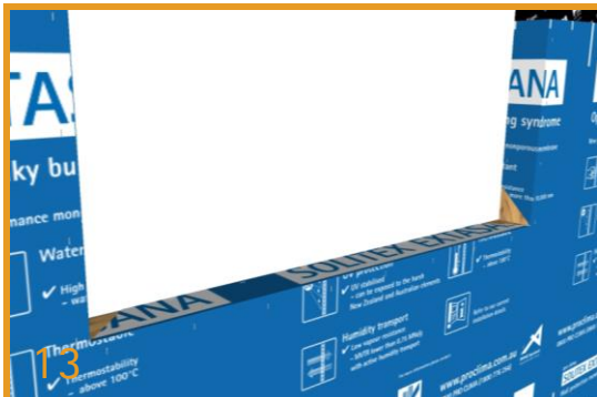
Sill Flashing – TESCON EXTOSEAL® Exposed framing at corners of the sill needs to be covered with TESCON EXTOSEAL® Sill Tape to prevent any leaks around windows entering the framing.
