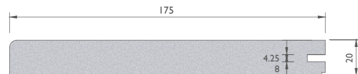
Lame de finition large 175 mm x 3150 mm x 20 mm
