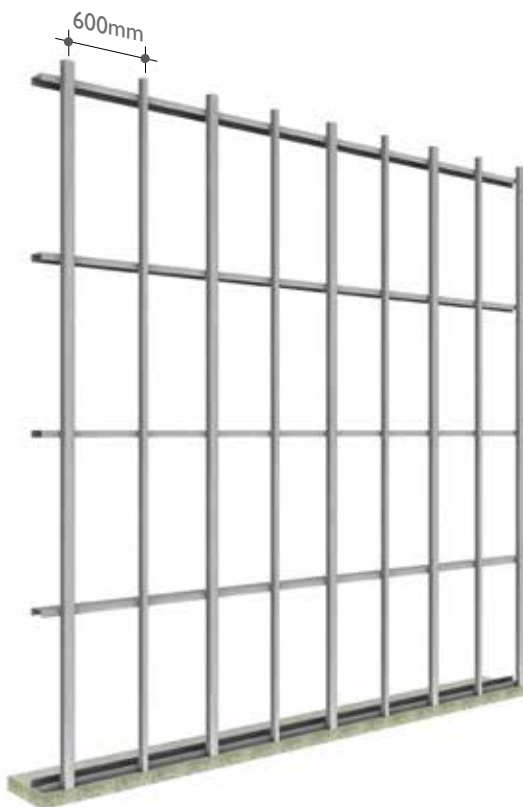
Figure 7 Direct fix to framing method
