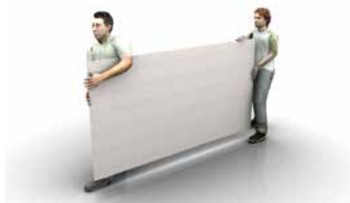
Figure 3 Always carry the board on edge but DO NOT store on edge
