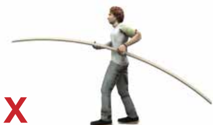
Figure 4 Never carry Kalsi cavity batten on flat and middle position, as this increases likelihood of breakage.
